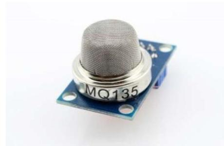
Fig 5: Gas Sensor MQ135
