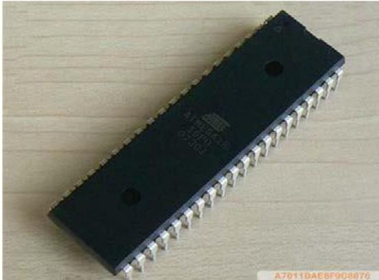
Fig 2: Atmega324A Microcontroller
