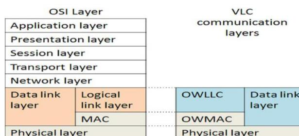
The essential layers in VLC OSI model is Physical Layer (PHY) and Data Link Layer (DLL). These are important for sending and receiving the light signal. The Media Access Control (MAC) and Physical layers are same for both transmitter and receiver part. [5]
