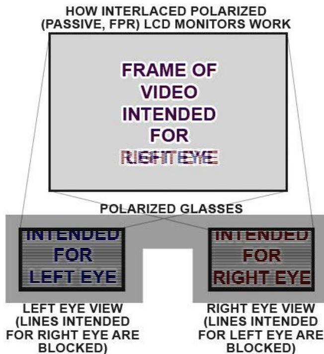
**Fig. 9 Working of Polarized Systems**
