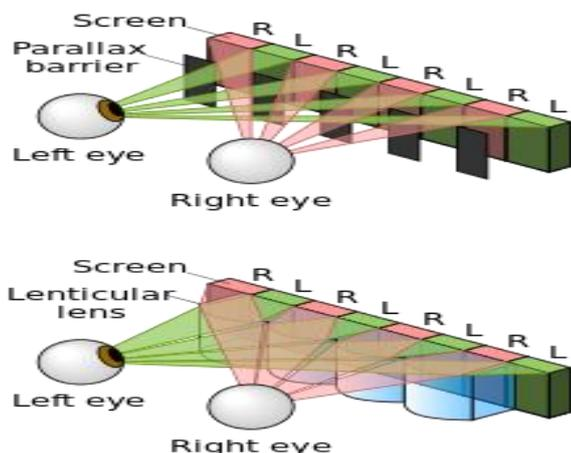
**Fig. 12 Comparison between parallax barrier and Lenticular displays.**
