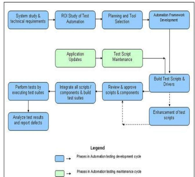
Fig. (3). Automation Testing Workflow [Adapted from <http://www.xoriant.com/>] [4]
