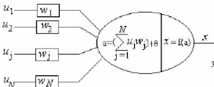
Fig. 1. Artificial Neuron Structure
