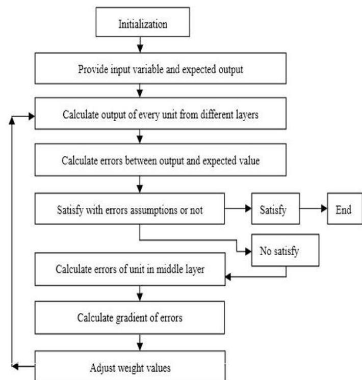
Fig. 3. Back Propagation workflow diagram
