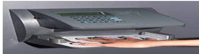
Physical security access management with a hand mathematics scanner
