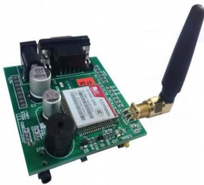
Fig.8 GSM Module
