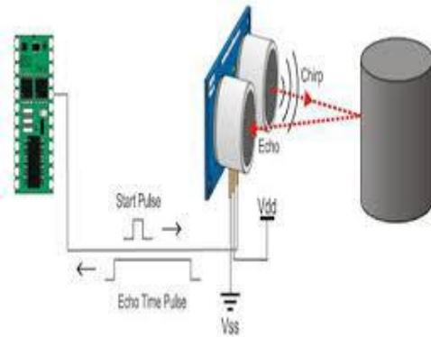
Fig.4 Obstacle detection circuit
