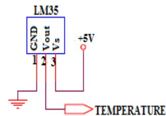
Fig.2 LM35 circuit
