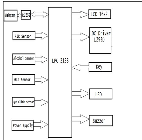
Fig. 1 Functional block diagram of the system.
