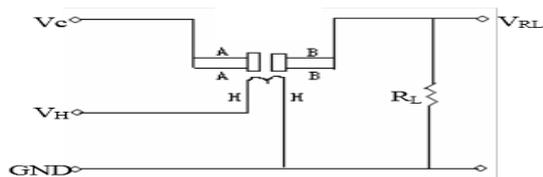
Fig. 6 Circuit Diagram of Gas Sensor
