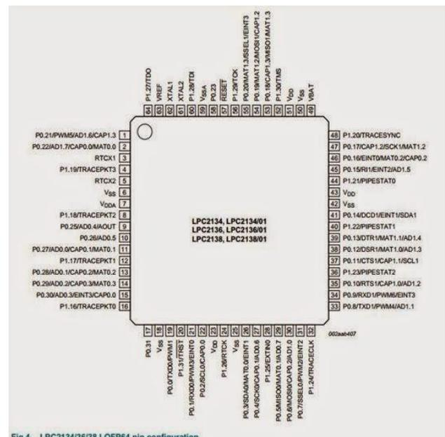
Fig. 2 LPC2138 Pin Configuration
