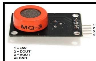
Fig. 4 Alcohol Sensor
