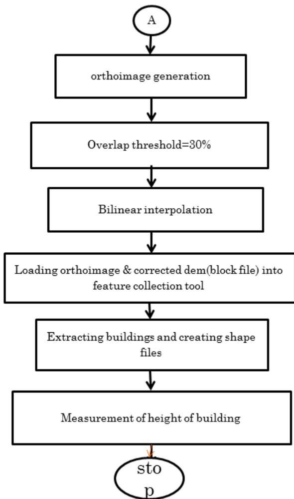
Fig. 2. Algorithm for building detection ,extraction and its height measurement from image from cartosat-1
