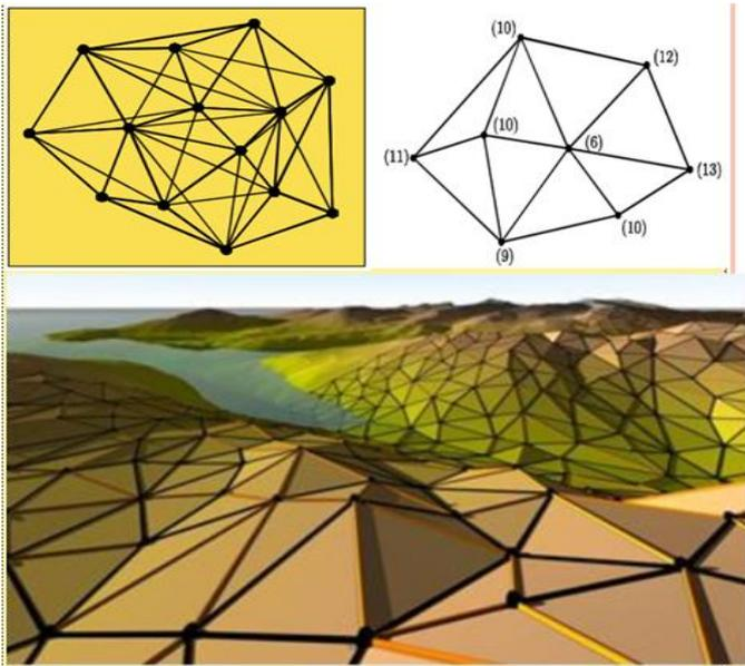
Fig.5. Triangulation representation of DEM
