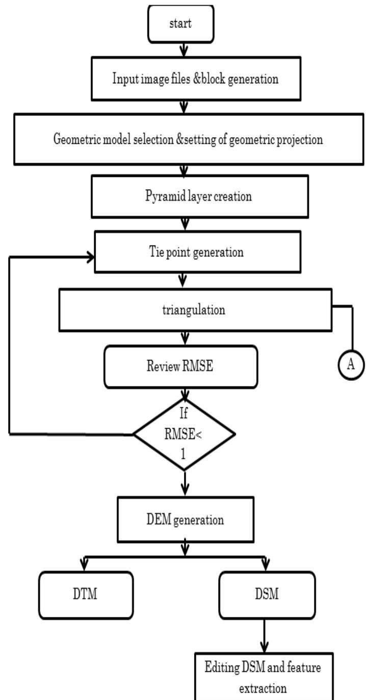
Fig. 2. Algorithm for building detection ,extraction and its height measurement from image from cartosat-1
