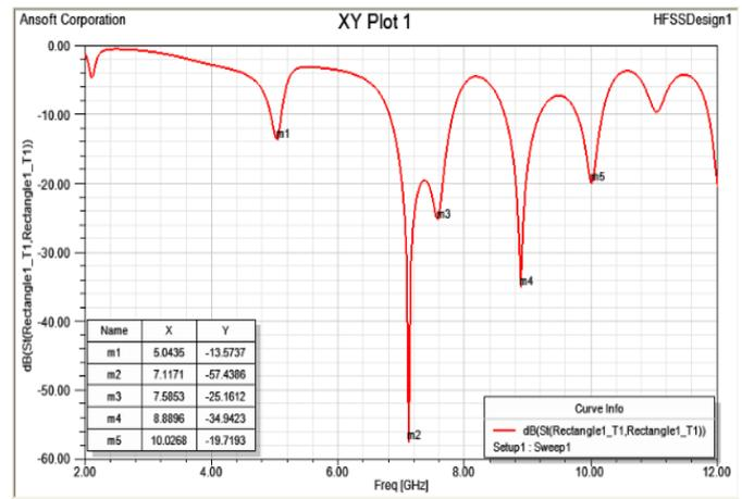
Fig.3. Return Loss at different frequencies
