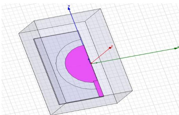
Fig. 2. Designed geometry for Circular – slot antenna
