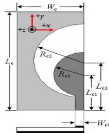
Fig.1. Geometry of proposed Circular – slot UWB antenna
