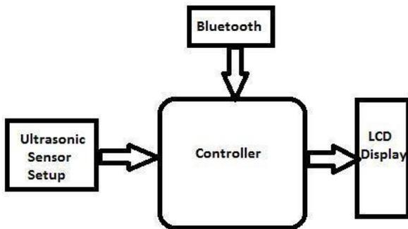
After ultrasonic waves were produced, ultrasonic transmitter transmits the ultrasonic waves toward a road surface to find out the obstacle. The range that obstacle detected is depends on the range of ultrasonic sensors that used. The ultrasonic wave detects any kind of physical obstacle, hence it will produce a reflected wave.
