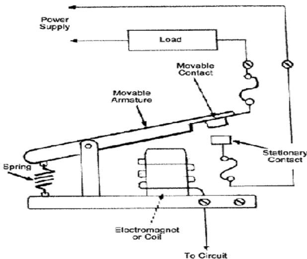
The first is at the bottom and drives the electromagnet. In this circuit, a switch is controlling power to the electromagnet. When the switch is on, the electromagnet is on, and it attracts the armature. The armature is acting as a switch in the second circuit. When the electromagnet is energized, the armature completes the circuit. When the electromagnet is not energized, the spring pulls up the armature away and the circuit is incomplete [5].
