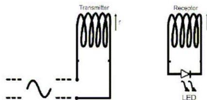
But this method is only for short distance transmission and has poor efficiency. For greater efficiency we need inductive coupling with many intermediate coils between transmitter and receiver.
