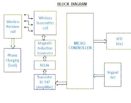
On the primary side, we have a primary coil whom we supply AC from the input power supply. Since the supply is DC, we first convert it to AC by using a rectifier.
