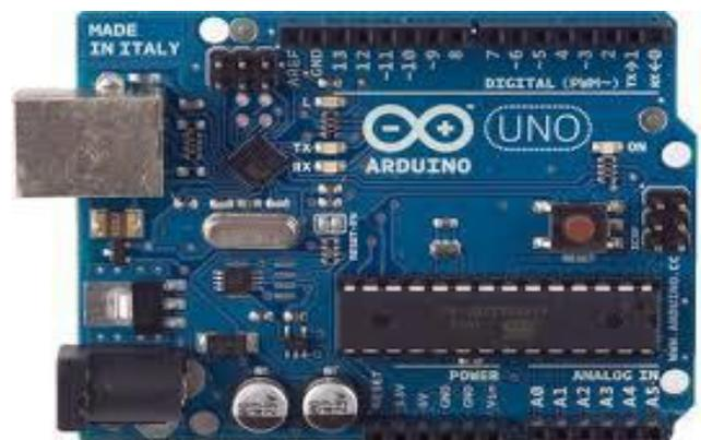
Fig:- Arduino Circuit Board with built in ATMEGA 328
