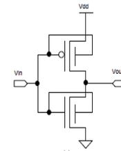
Fig.2 Inverter using FinFET in SGmode
