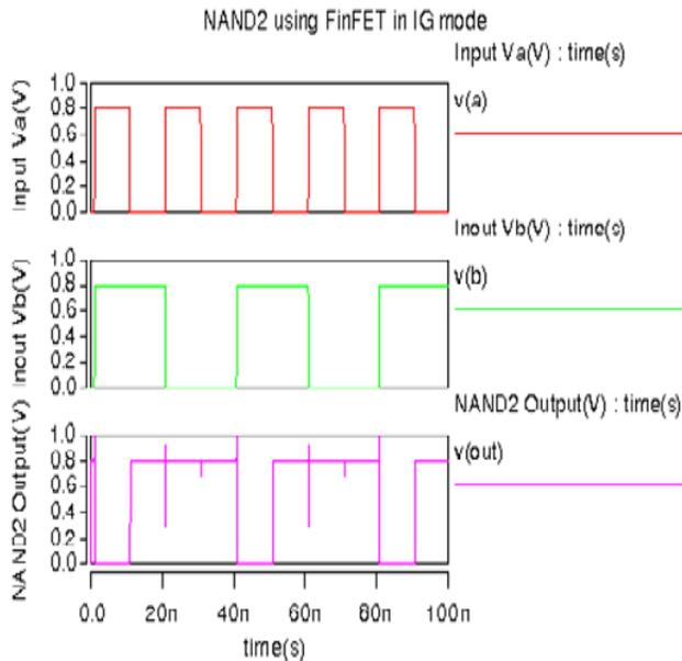
Fig.9 Waveforms for NAND2 using FinFET (IGmode)
