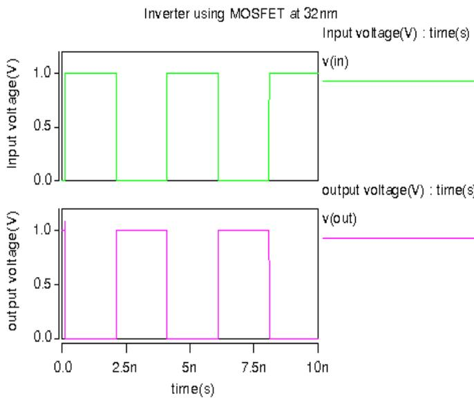
Fig.5 Waveforms for MOSFET based Inverter using 32nm
