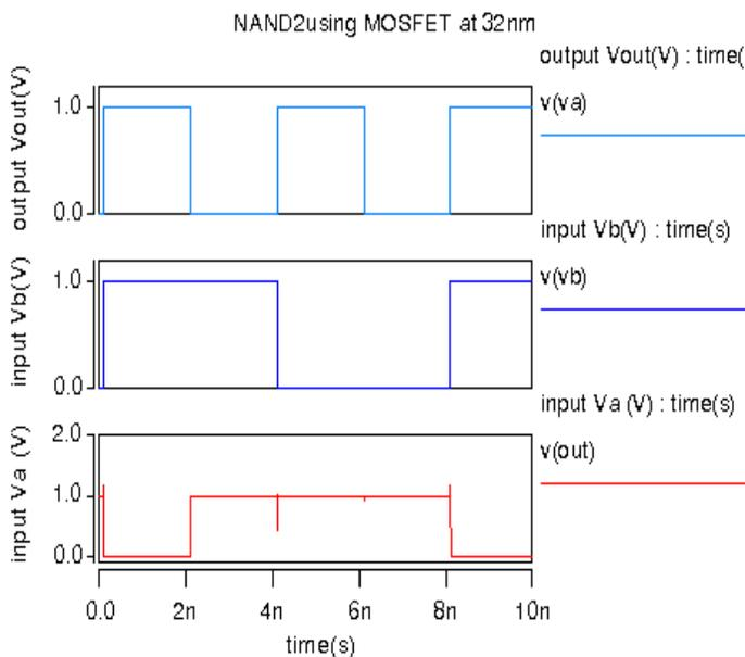
Fig.6 Waveforms for MOSFET based NAND2 using 32nm
