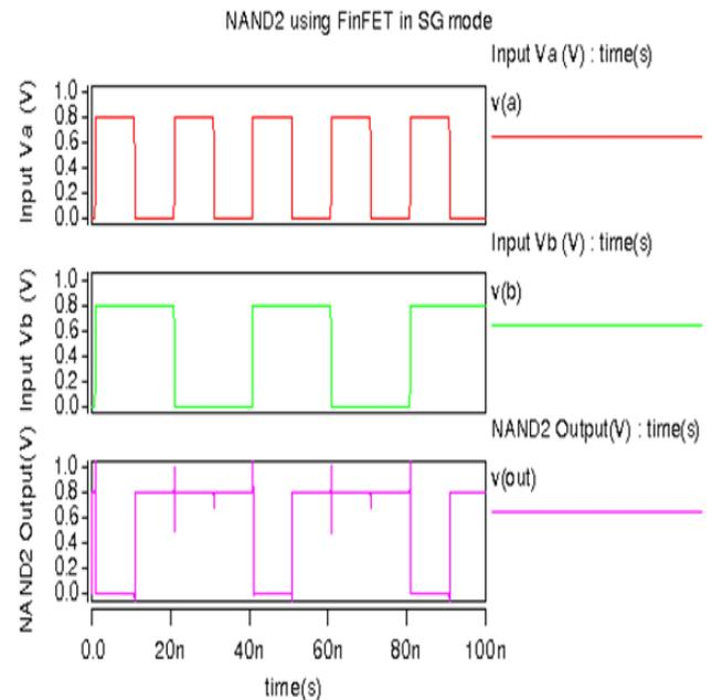
Fig.8 Waveforms for NAND2 using FinFET (SGmode)
