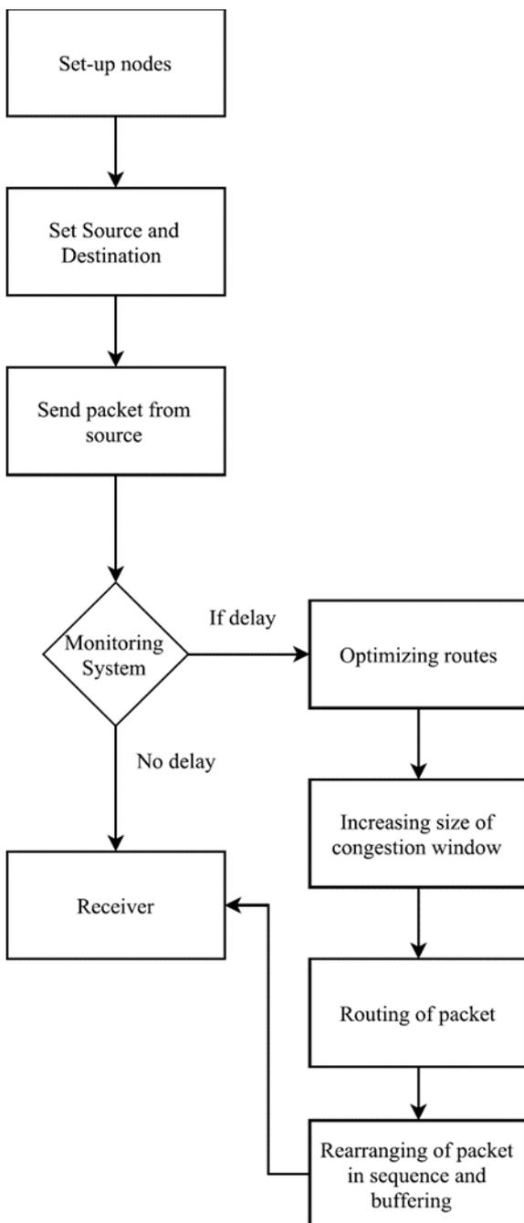
Fig 2- Architecture Diagram
