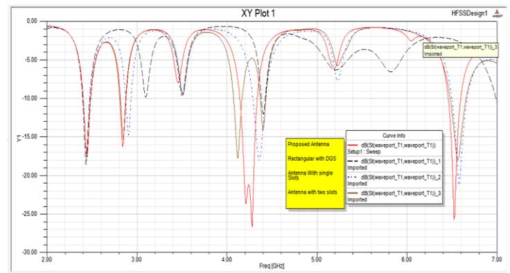
Figure 4: Return loss Vs Frequency curve for designs
