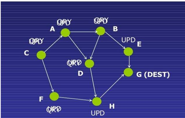
Fig. 7. Route Maintenance in TORA
