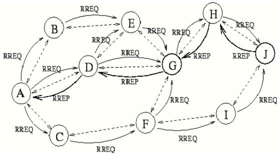
Fig. 4: Route Request and Route Reply in AODV
