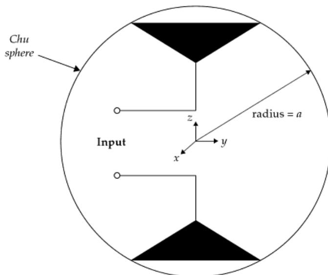
Fig-3, An Electrically small antenna, the largest dimension of the antenna are enclosed within the sphere of radius a.
