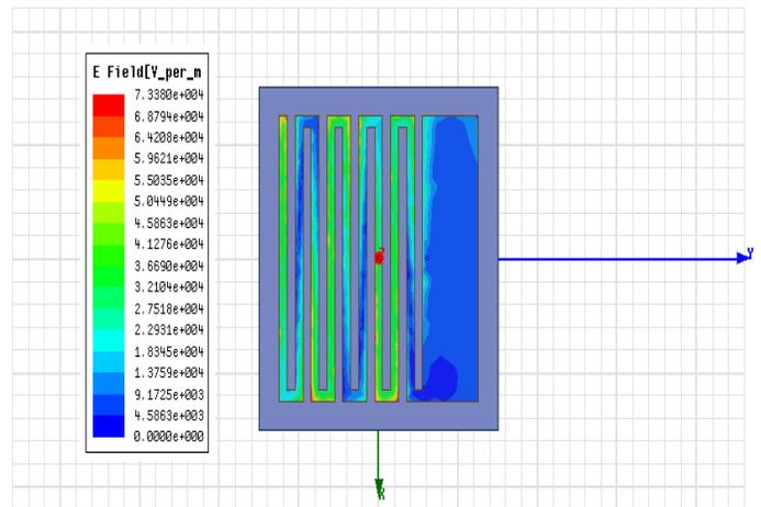
Fig-7 plot of Electric field intensity (V/m) of electrically small antenna
