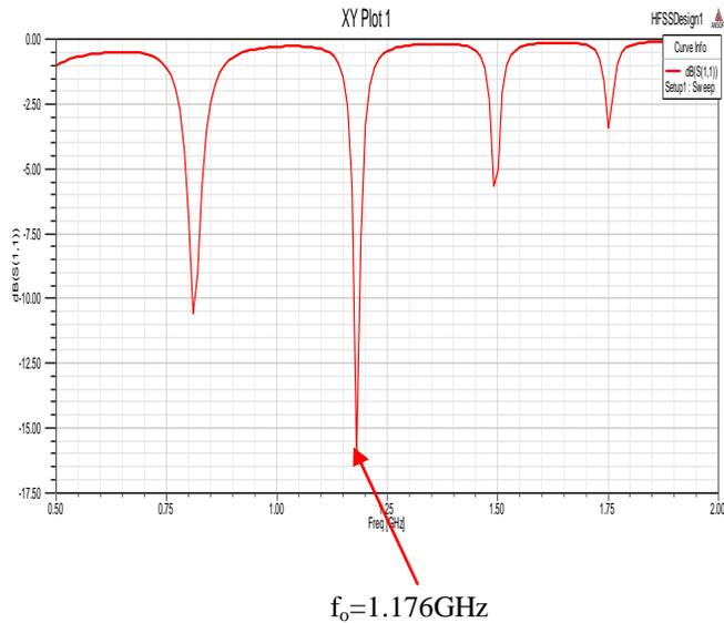
Fig-5, Return loss (S11) of the Meandered ESA.
