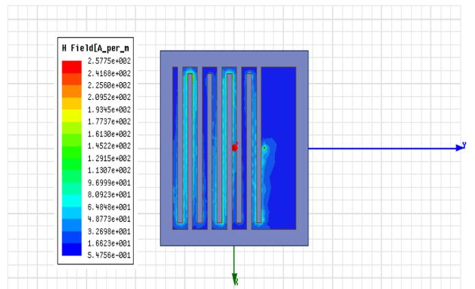
Fig-8 Plot of Magnetic field intensity (A/m) of electrically small antenna
