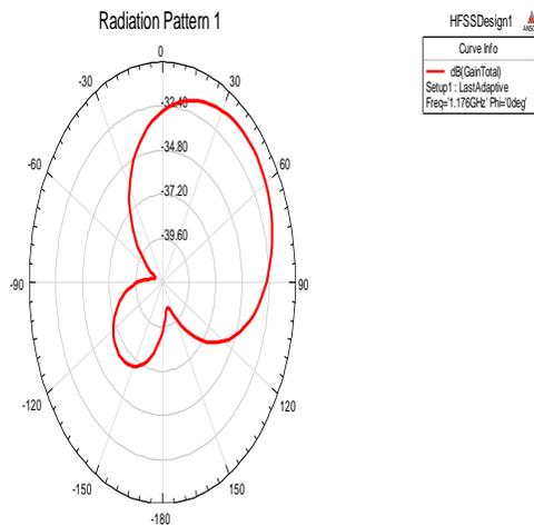
Fig-9, Radiation Pattern Of the Meandered Line Patch Antenna.
