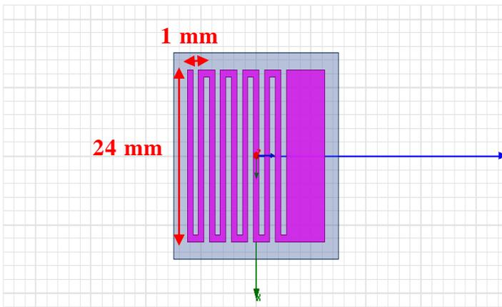
Fig-4, Top view of the proposed design of electrically small antenna.
