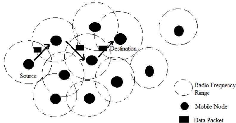
Figure: - 1 Mobile Nodes sending the Data Packet in a Multi-hop Fashion
