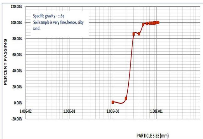
Fig 1.0: Particle Size Distribution Curve
