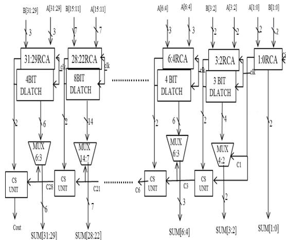
Fig. 6 32-bit CSLA using D latch
