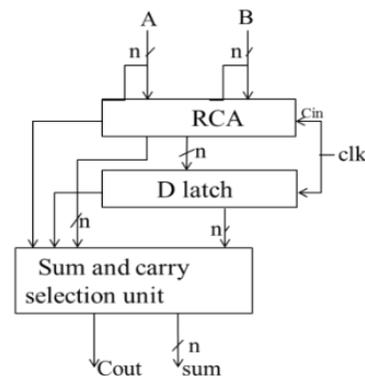
Fig. 5 CSLA using D latch
