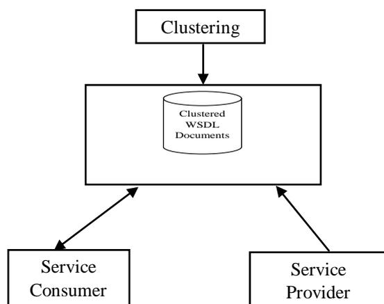
Fig.1 Proposed architecture of web service clustering
