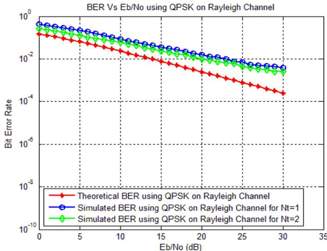
**Fig. 8 BER Vs Eb/No FOR QPSK**
