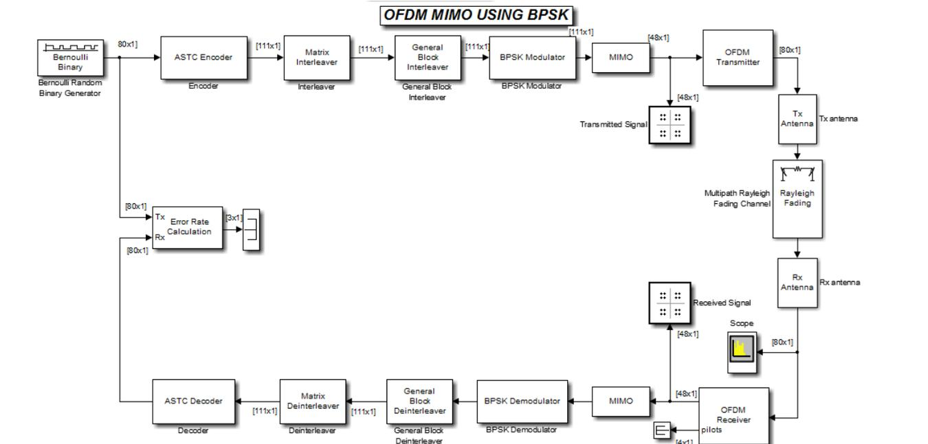
**Figure 2. Proposed Model of MIMO OFDM.**
