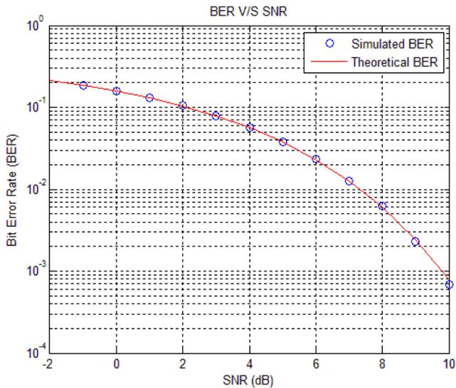
Fig. 4 BER Vs SNR FOR BPSK
