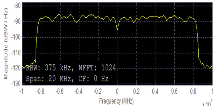
Fig. 6 QPSK signal FREQUENCY response of multipath Rayleigh fading channel
