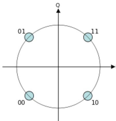
Figure 1. Constellation diagram for QPSK
