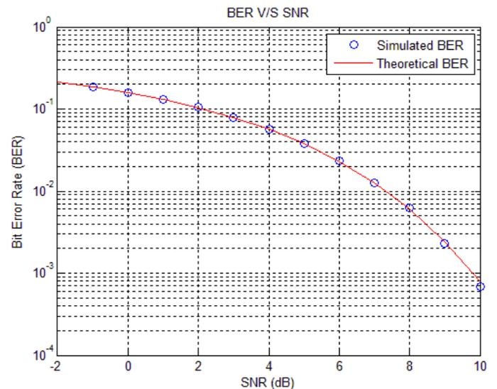
Fig. 7 BER Vs SNR FOR QPSK
