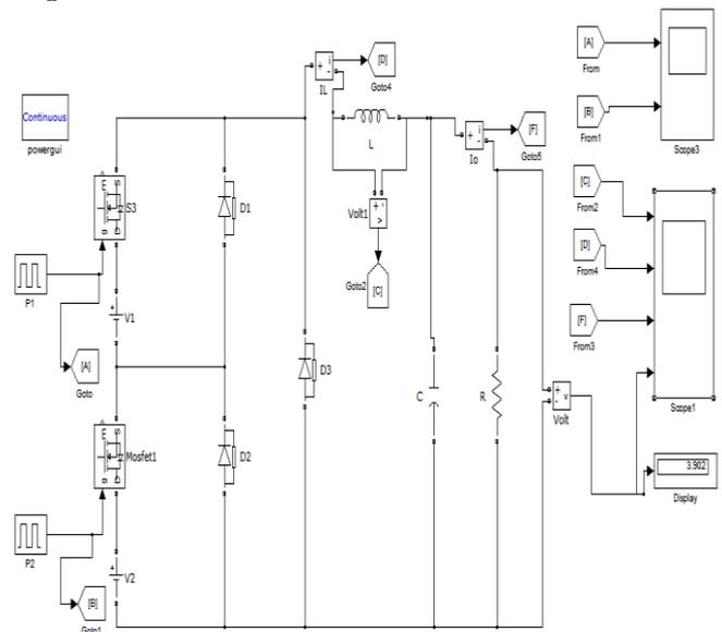
Fig.7.Simulation model of dual input buck-buck converter using MATLAB
