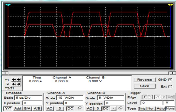
Fig.11.Switching signals of dual input buck-buck dc-dc converter using MULTISIM
