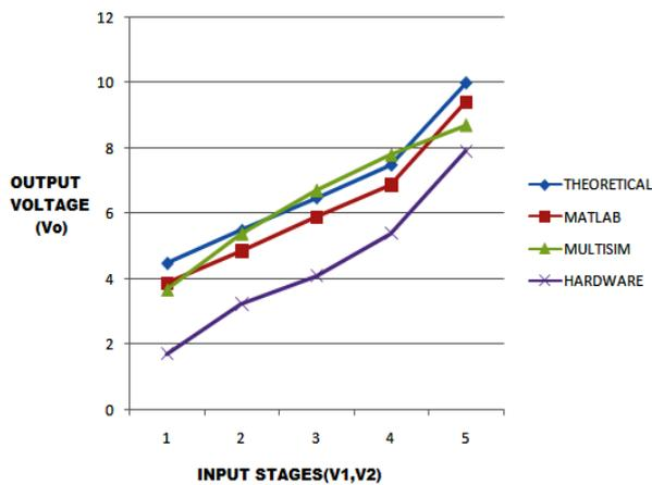
Fig.15. Output voltage Comparison of dual input buck-buck dc-dc converter
