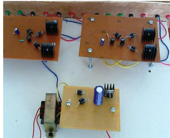
Fig.13. Hardware model of dual input buck-buck dc-dc converter
