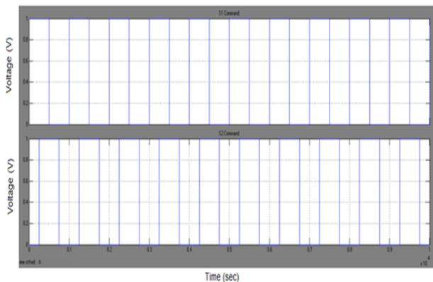
Fig.8 .Switching signals of dual input buck-buck dc-dc converter using MATLAB
