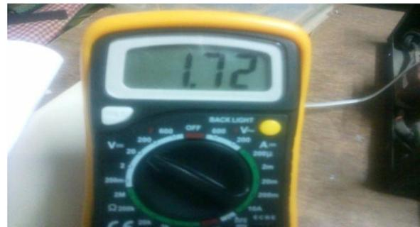
Fig.14.Hardware Output voltage of dual input buck-buck dc-dc converter
