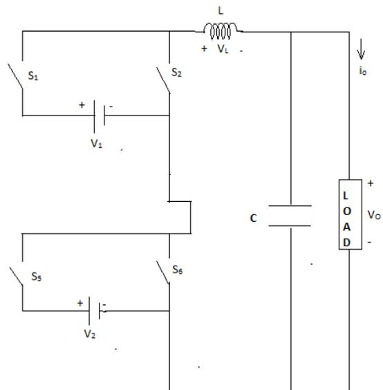
Fig.4 Final stage of dual input buck-buck converter using H-bridge cells
