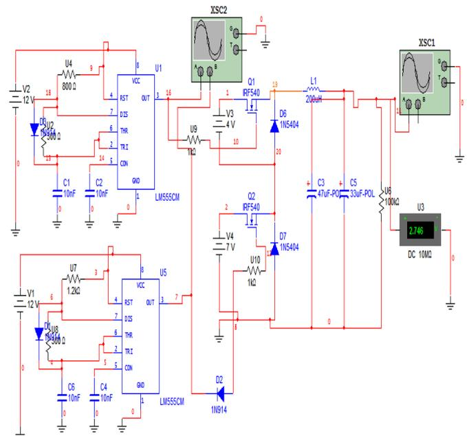
Fig.10.Simulation model of dual input buck-buck dc-dc converter using MULTISIM
