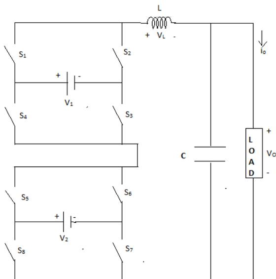
Fig.3 First stage of dual input buck-buck converter using H-bridge cells
