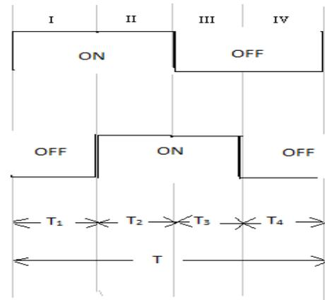
Fig.6 .Switching pattern of dual input dc-dc converter
