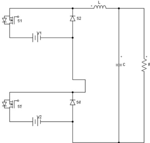
Fig.5..Circuit diagram of dual input buck-buck converter using H-bridge cells
