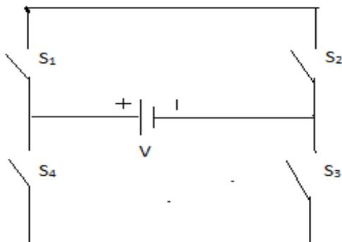
Fig.2.Circuit diagram of an H-Bridge cell.
