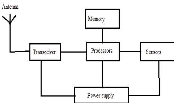
Figure 1: Sensor Node Architecture
