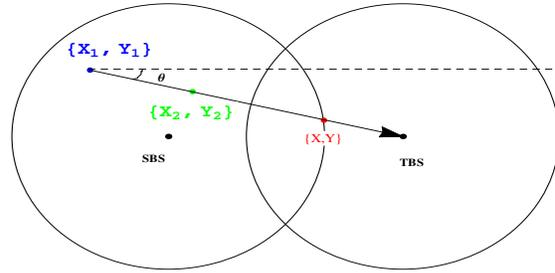
Fig. 3. A MS leaving its SBS and moving toward a TBS.
