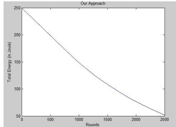
Fig. 6. The total energy of WSN during each round
