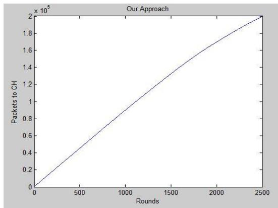
Fig. 5. The total number of packets sent to cluster-head during each round
