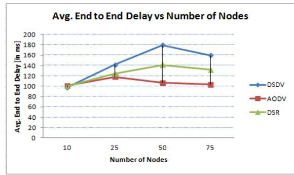
Figure 3(d): Average End to End Delay vs. varying No. of Nodes
