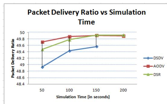
Figure 2(c): Packet Delivery Ratio vs. varying Simulation Time
