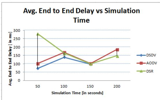
Figure 2(d): Average End to End Delay vs. varying Simulation Time
