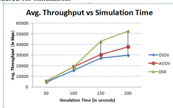
Figure 2 (a): Average Throughput vs. varying Simulation Time
