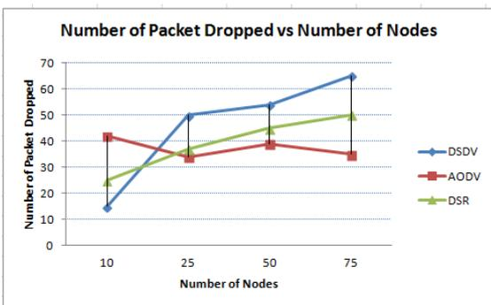
Figure 3(b): Number of Packet Dropped vs. varying No. of Nodes
