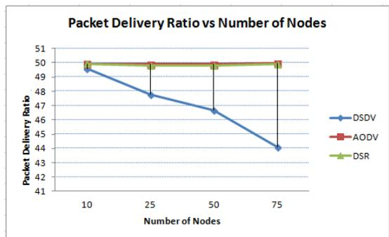
Figure 3(c): Packet Delivery Ratio vs. varying Number of Nodes
