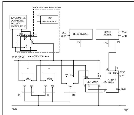
Figure 2: Schematic of RFID Door Locking System
