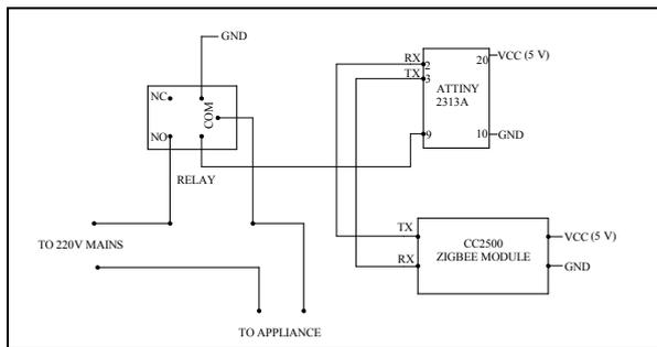
Figure 4: Schematic of Wireless Switch
