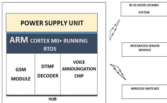
Figure 1: Basic block diagram of Gateway
