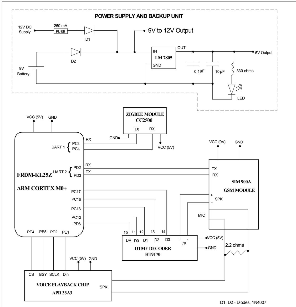
Figure 13: Complete schematic of HUB
