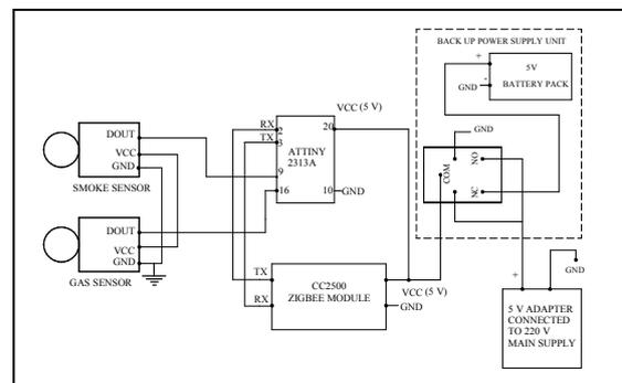
Figure 3: Schematic of Integrated Sensor Module
