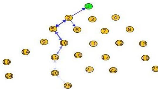
Figure 3 RPL DODAG generation, 1 sink node and 24 sender nodes
