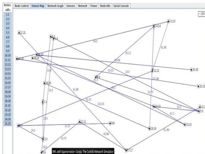
Figure 2 Topology of a WSN with 25 nodes.
