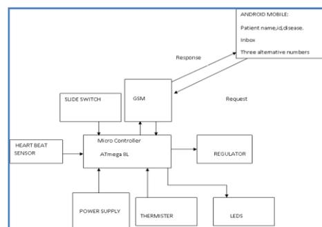
Fig 3.1 Structure flow chart
