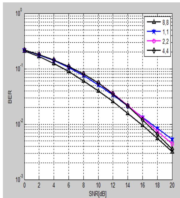
Fig. 6. Simulation results of Sphere Decoding
