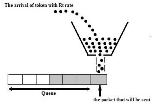
Fig. 5 token bucket mechanism
