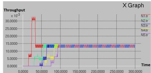
Fig.10 The behavior of the bandwidth occupied by each node with the FGMA algorithm while the simulation
