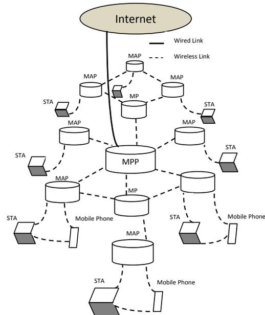
Fig. 1 Architecture of a wireless mesh network
