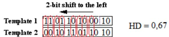
Fig -7: Example of calculating the Hamming distance (HD) with one step shift of iris bit templates
