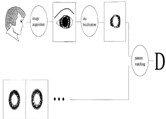
Fig -4: Schematic diagram of iris recognition system
