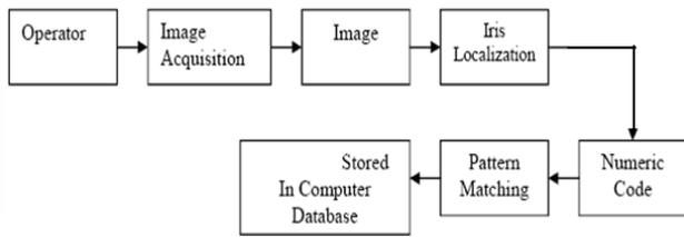
Fig -2: Block diagram of iris recognition system
