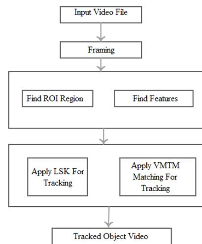
Fig. 1. Architecture Diagram
