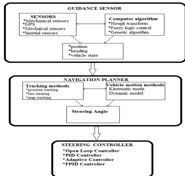
Fig. 5: Framework of agricultural vehicle autonomous guidance system
