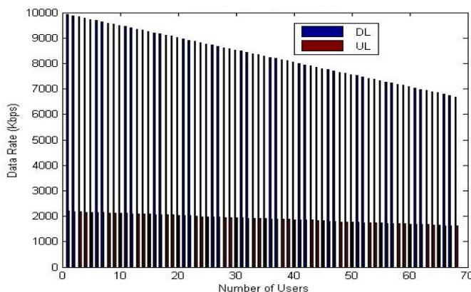
Fig.12: DL/UL Capacity of WiMAX
