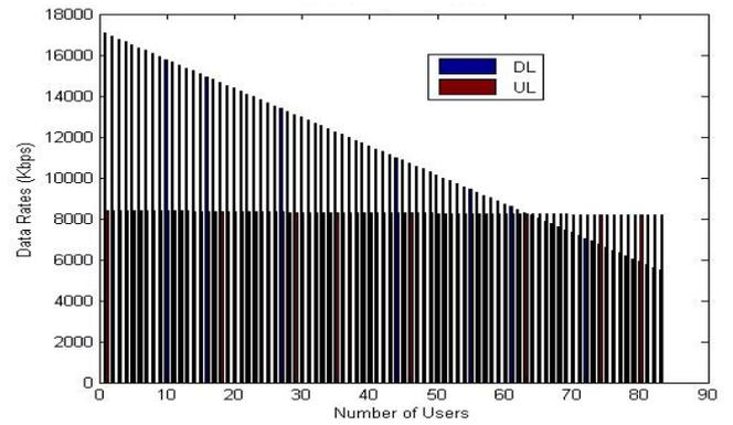
Fig.9: DL/UL Capacity of LTE
