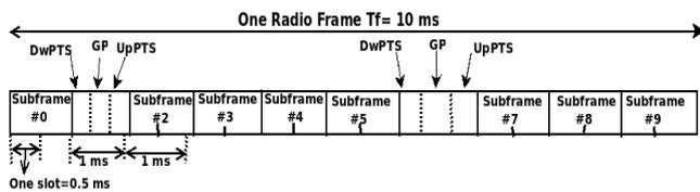
Fig.3: LTE Frame Structure
