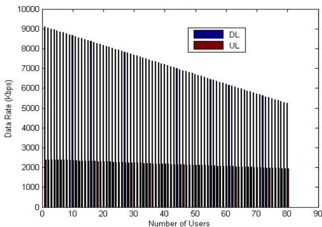
Fig.8: DL/UL Capacity of WiMAX
