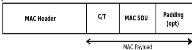
Fig.4: MAC PDU Structure of LTE
