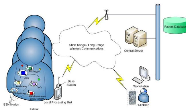
Fig.1.1: Schematic diagram Body Area network
