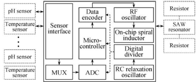
Fig.: 3.1. Schematic diagram of the system-on-chip architecture.
