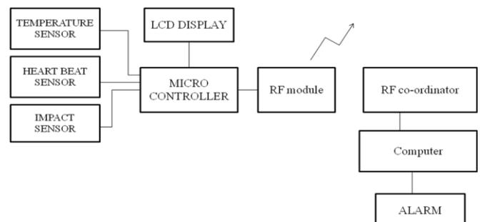
**Fig.: 4.1. Proposed system block diagram**
