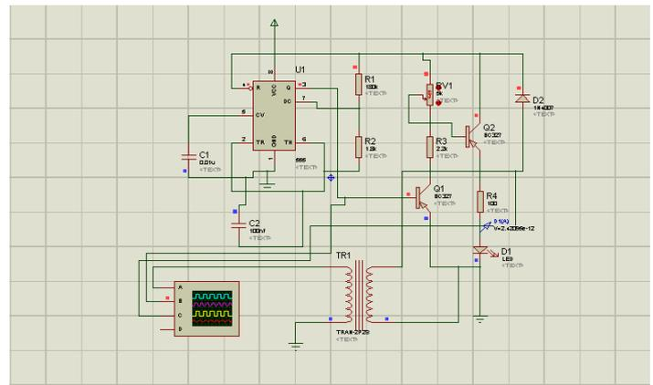
Fig.11 Simulation of PWM and voltage sources
