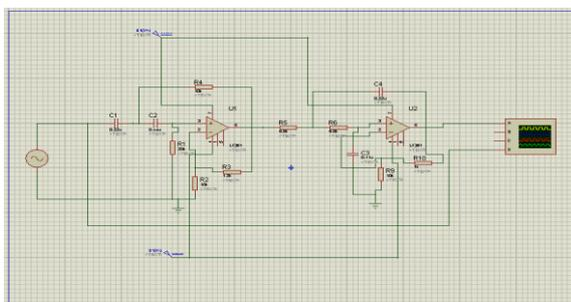
Fig. 1 Design of Butterworth Band pass filter
