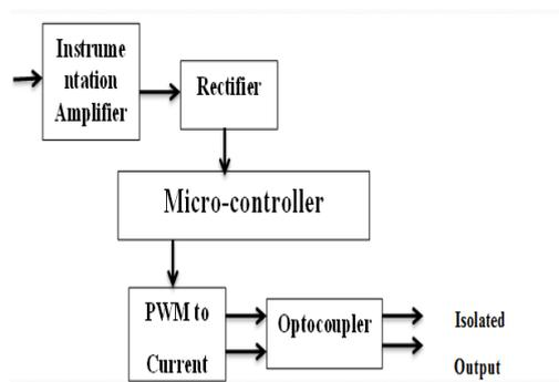
Fig.8 General Functional block diagram of Stimulator
