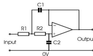
Fig.4 Operational amplifier two pole low pass filter
