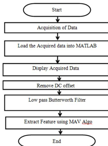
Fig.7 Flowchart for MES Feature extraction
