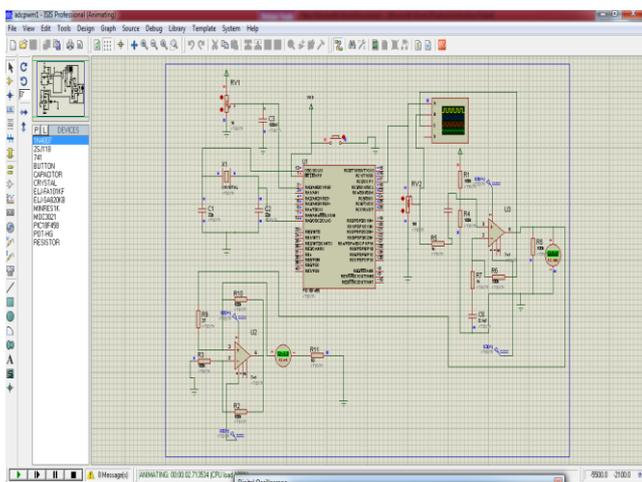
Fig.9 Simulation of PWM and current source
