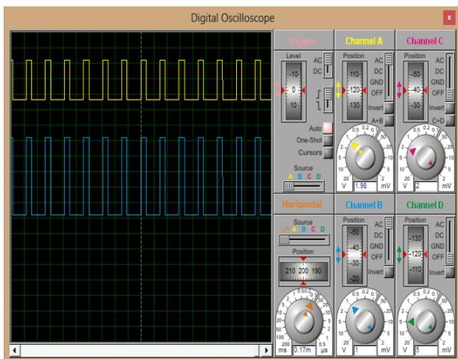
Fig.10 Output of simulation of PWM for continuous pulses
