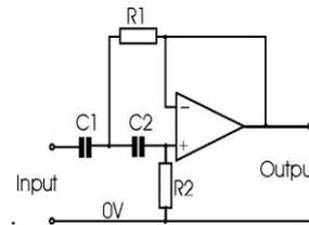
Fig.3 Operational amplifier two pole high pass filter
