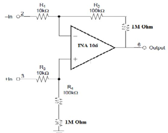
Fig.2 Design of Instrumentation amplifier
