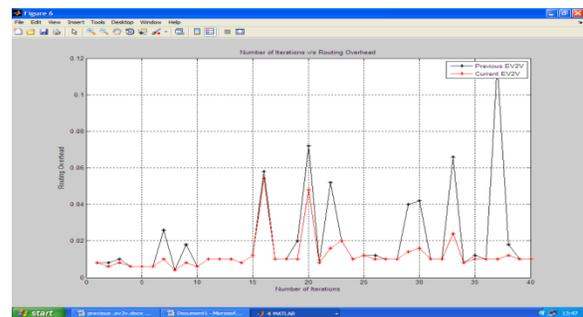
Figure shows the comparison of the previous effective vehicle to vehicle communication protocol with the current effective vehicle to vehicle communication protocol for vanets by using the parameter with respect to the routing overhead.
