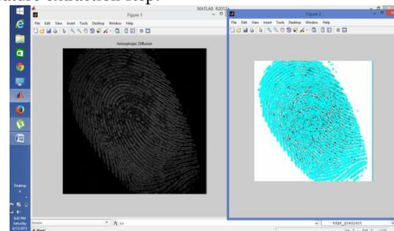
Figure 1: Fingerprint enhanced using anisotropic diffusion.
