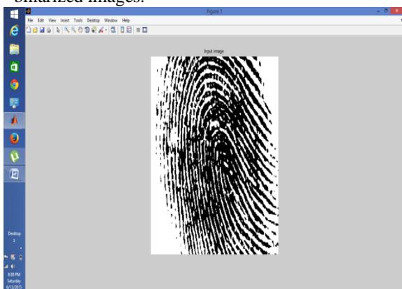
**Figure 3:** Output obtained after the binarization of the fingerprint impression.
