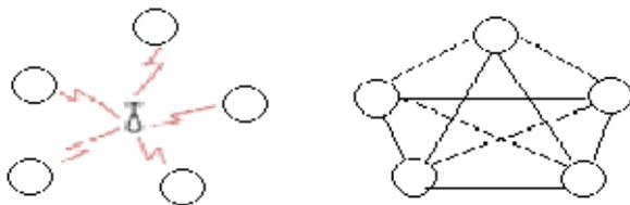
Figure 1. Centralized network (left) versus ad hoc network (right)
