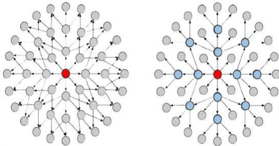
Figure 2: Broadcasted network, and the network with MPRs in OLSR.
