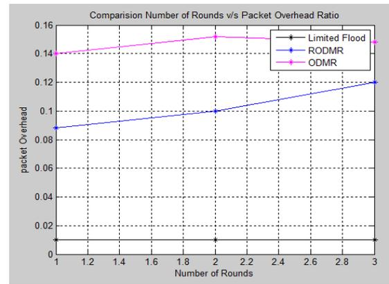
Fig.7: Packet overhead v/s number of rounds.
