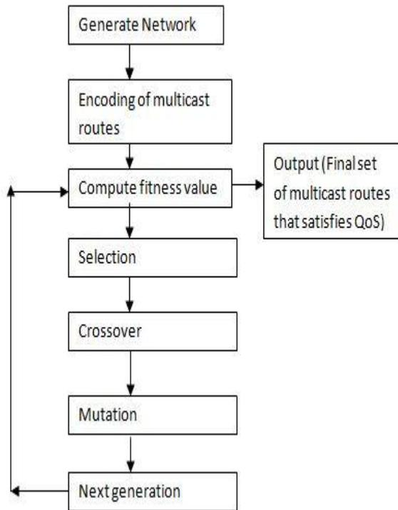
Figure. 3. Genetic Algorithm for QoS multicast routing.
