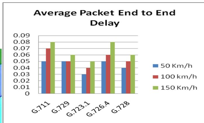
**Figure 3.10 Mean Packet end to end delay without Silence Suppression**
