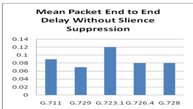
**Figure 3.4** Average packet end to end delay without Silence Suppression
