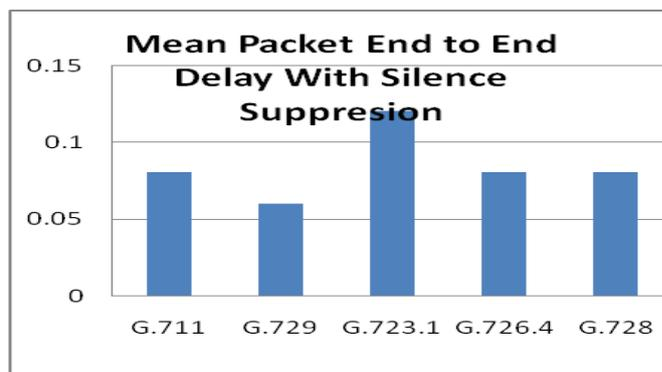
**Figure 3.5** Average packet end to end delay using Silence Suppression
