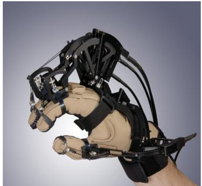
Fig. 2.2 Haptics Feedback device
