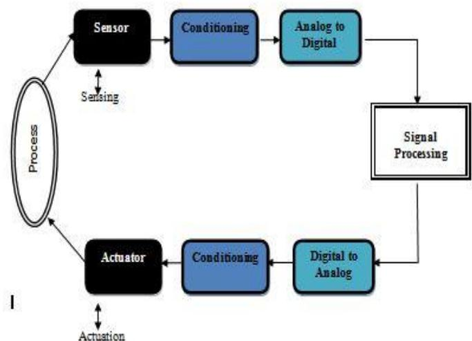
Figure 1.1 Data acquisition and actuation
