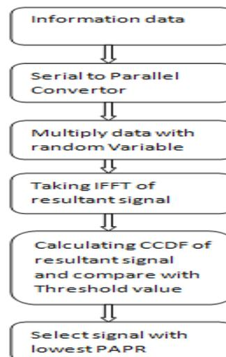
Fig. 2 Flow chart for SLM technique.
