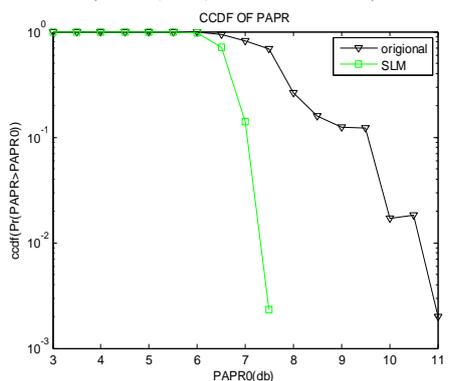
CCDF of SLM PAPR and original scheme M=16 Sub-blocks (N=256, L=4, BPSK modulation)
