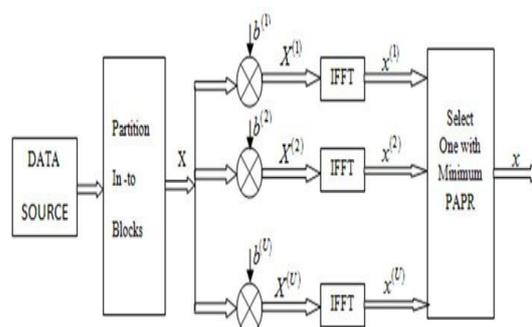
Fig. 2 Block Diagram of Selective mapping technique
