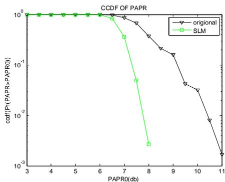
CCDF of SLM PAPR and original scheme with M=8 Sub-blocks (N=256, L=4, BPSK modulation)
