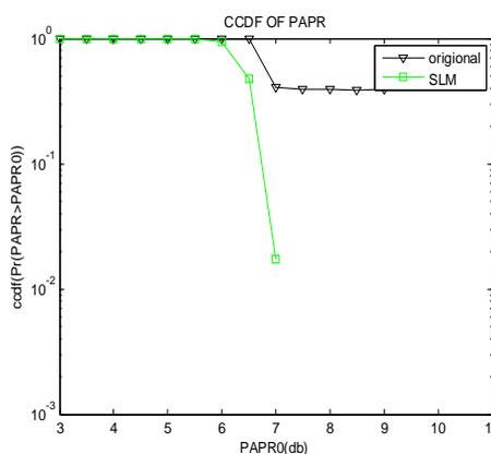
CCDF of SLM PAPR and original scheme with M=32 Sub-blocks (N=256, L=4, BPSK modulation)
