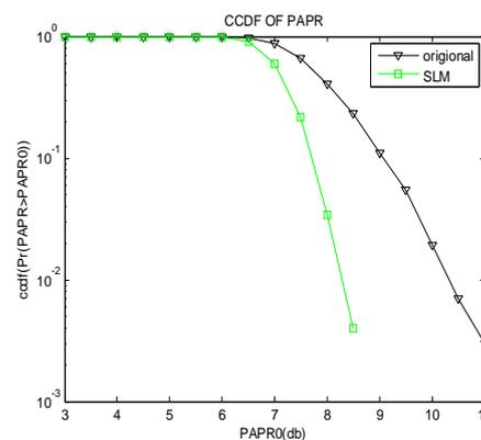
CCDF of SLM PAPR and original scheme with M=4 Sub-blocks (N=256, L=4, BPSK modulation)
