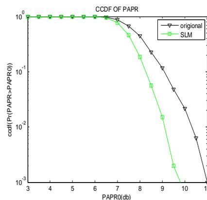
CCDF of SLM PAPR and original scheme with M=2 Sub-blocks(N=256,L=4,BPSK modulation)
