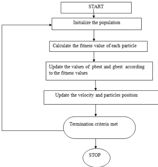
Figure 4.4: Flowchart of the PSO Algorithm
